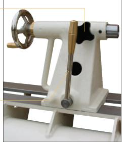
**Installation of Accessories:** To install an accessory in to the tailstock, wind the barrel out 1". Put the accessory in the barrel, and snap it into the taper.
