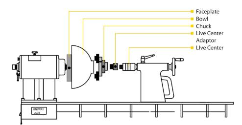
both assure clearances of toolrest, bed, etc. as well as assuring that chuck keys or wrenches have been removed.
